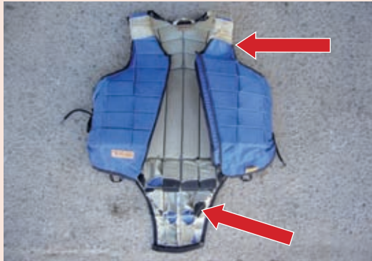
Body protector – damaged with excessive wear.
