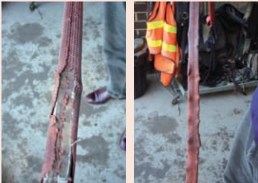
Riding reins – damaged and worn.
